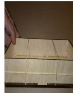
9. Glue notches on top of piece and edges
